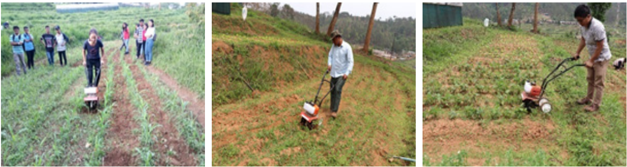
Fig 16. Field testing of mini-tiller for weeding operation on terraces
