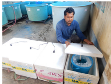
Fig 27 (B). CT max and CT min assessment in polystyrene boxes using thermostats
