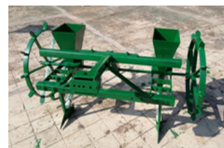
Fig 24 (b). Developed sowing attachment
